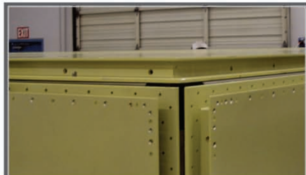
Close up of Predetermined Holes on Panel Edge Members and Closeouts
