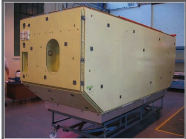
A fuel tank undergoing First Article Inspection
